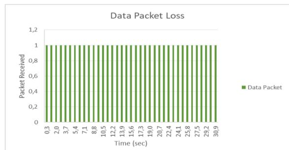
Figure 4 - High data rate- Shopping busy hours – Data packet loss
