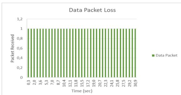
Figure 1 - High data rate- Ideal – Data packet loss
